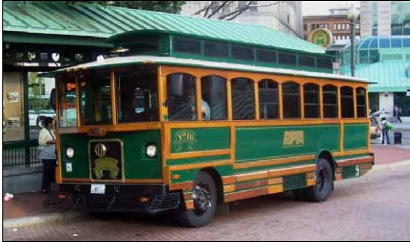
A tourist trolley, also called a road trolley, is a rubber-tired bus, which is made to resemble an old-style streetcar. The name refers to the American English usage of the word trolley to mean an electric streetcar. As these vehicles are not actually trolleys, and to avoid confusion with trolley buses, the American Public Transportation Association (APTA) refers to them as "trolley-replica buses"
