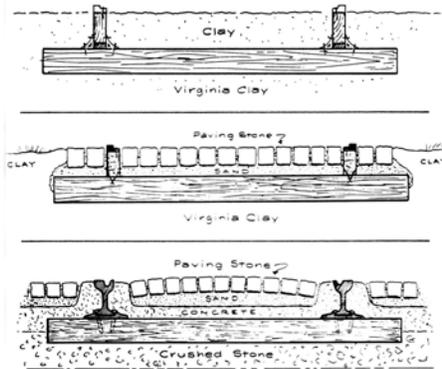
Streetcar tracks were laid in the same way as railroad tracks. Steel rails were spiked to wood ties. These were below the street level. The cavity was filled so that the top of the tracks were flush with the street. This prevented people from tripping on them.
